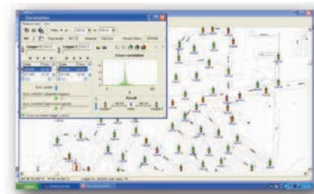
Acoustic data from loggers placed on valves or hydrants along the water main is correlated, allowing identification of potential leak locations.
